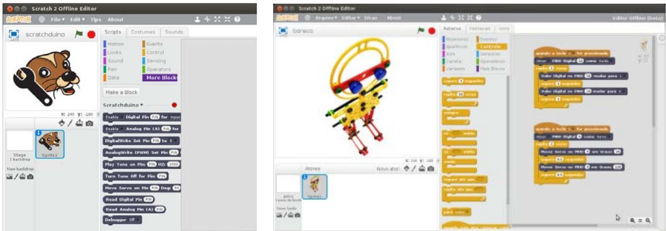
Figure 3. s2a\_fm blocks used by Scratchduino and example of Scratch program for moving the robot's arm
